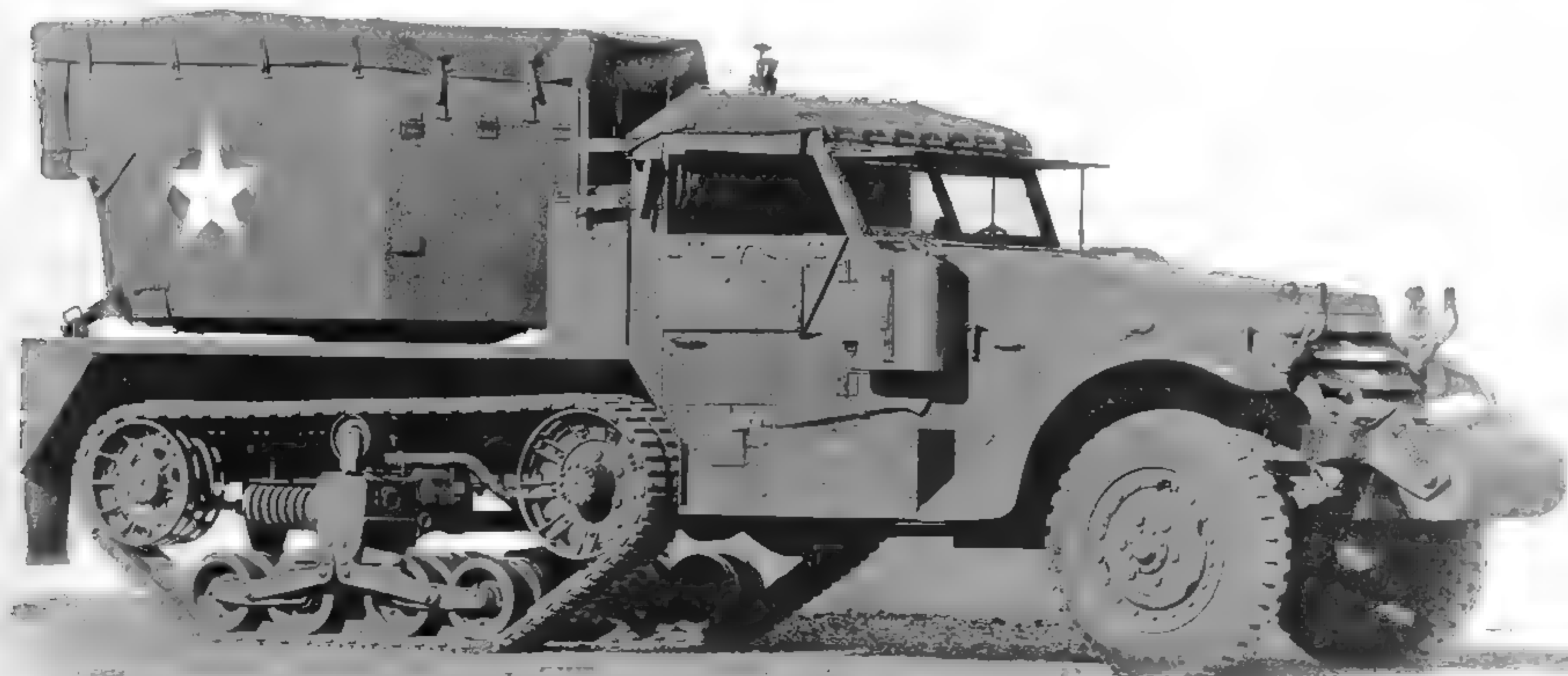
This new Autocar M15A1 Multiple Gun Motor Carriage was photographed at the Studebaker Proving Grounds. The demountable headlights and unditching roller are plainly visible, as are the unusual canvases protecting the gun mount and driver's compartment. (U.S. Army photo)
